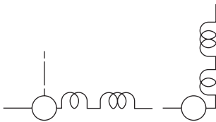
46.8.5 Direct-current series motor or 2-wire generator; with commutating or compensating field winding or both*
